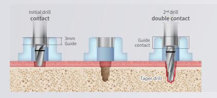
Initial Drill: The smart design assists the drill barrel for a fitted insertion to the guide sleeve up to 3mm prior contact with the bone.
