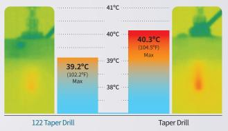
Drill temperature comparison between the 122 taper drills and other taper drills
