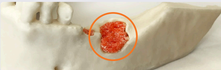
Once hydrated, it becomes moldable and can take the shape of a variety of defect shapes and sizes
