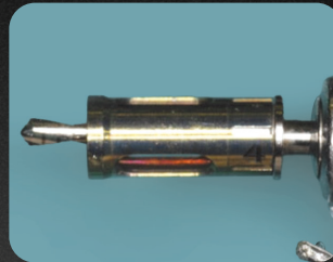
Ø2.2 Twist Drill with 4.0 mm stopper
