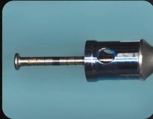
Depth gauge with 9.0 mm stopper
